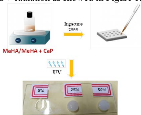
Figure 1: Photocrosslinking of nanocomposite MeHA/MaHA + CaP
