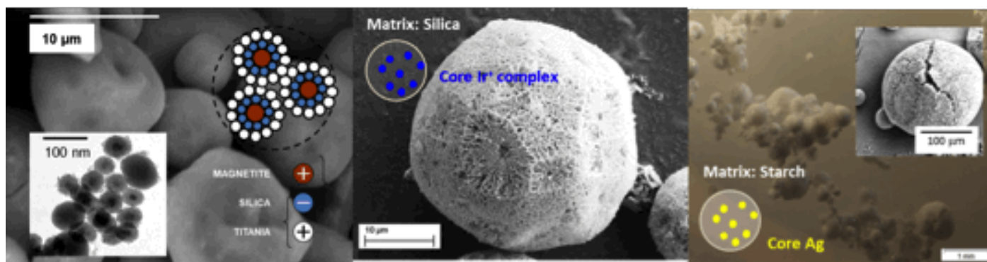
Micro-engineered capsules used as a) photocatalyst; b) luminescent materials; c) carrier of potentially hazardous nanoparticles.
